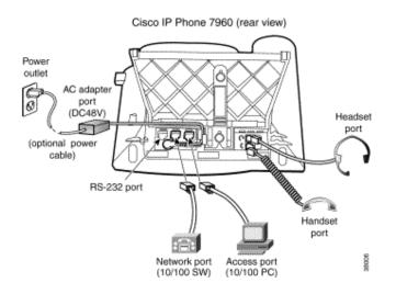
Figure 1: Cisco SIP-based IP Phone 7960 (rear view)<sup>3</sup>
