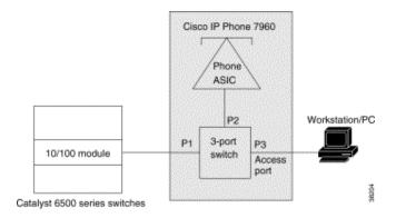
Figure 2: Switch-to-Phone Connections<sup>5</sup>
